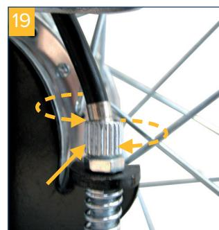
For adjustment, first remove the locking nut and then perform the corresponding adjustment; thereafter retighten the locking nut and in doing so, use pliers to hold the adjusting screw. To brake the wheelchair by the attendant, pull up both brake handles at the hand grip.
