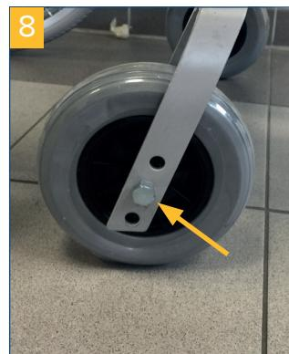
The plugs of the corresponding holes can be easily exchanged. Now move the wheel in the desired position and reinsert the wheel axle screw and tighten it (**photo 8**).
